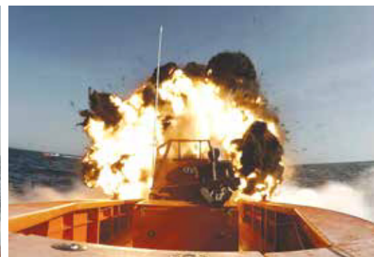
The FIAC's view of a JAGM moments before impact. Because of the significant horizontal and vertical movement associated with a small boat moving through choppy seas, traditional laser-guided missiles would be limited by the designator's ability to maintain a consistent laser spot and backscatter from sea spray.
