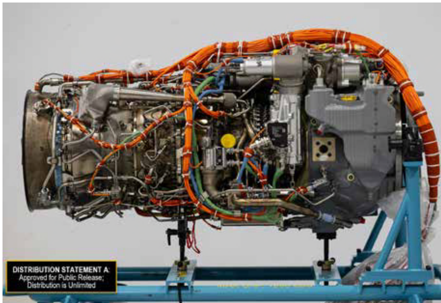
GE Aerospace T901 flight test engine designated for Future Attack Reconnaissance Aircraft (FARA) Competitive Prototypes.
