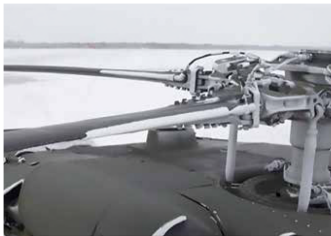
Ice accretion on UH-60 rotor blade.
