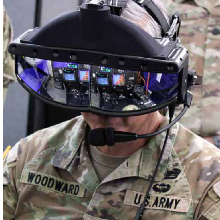
COL Scott Woodward, deputy commanding officer, U.S. Army Combined Arms Center – Training, examines the features of the Reconfigurable Virtual Collective Trainer-Aviation (RVCT-A) for the Army's Apache helicopter platform.
