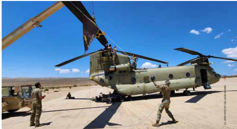
Co. B, 2nd Bn., 227th Avn. Regt. removes CH-47 main rotor blade to replace leaking seal during National Training Center Rotation 23-08. National Training Center, California June 22, 2023.
