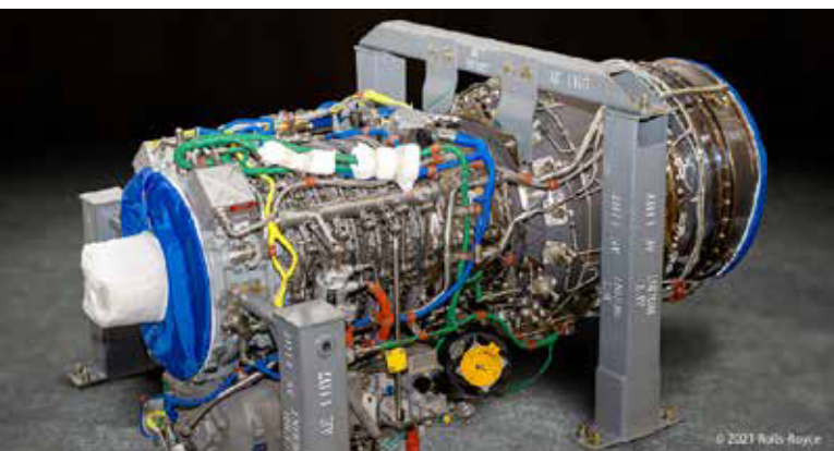
The Rolls-Royce AE 1107 engine powers the V-22 aircraft and will power the Bell V-280 aircraft competing for the Army's FLRAA program.
