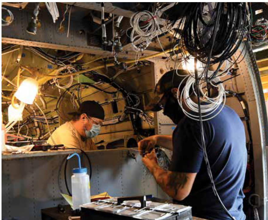
CCAD aircraft electricians Mike Lee (left) and Jonathan Lopez (right) work on installing the electrical wiring harness on a UH-60V.
