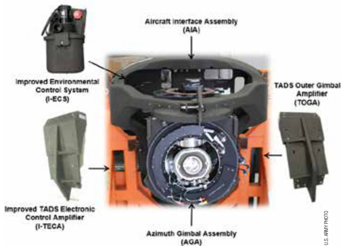
The new components will increase operational availability and boost system performance for pilots.
