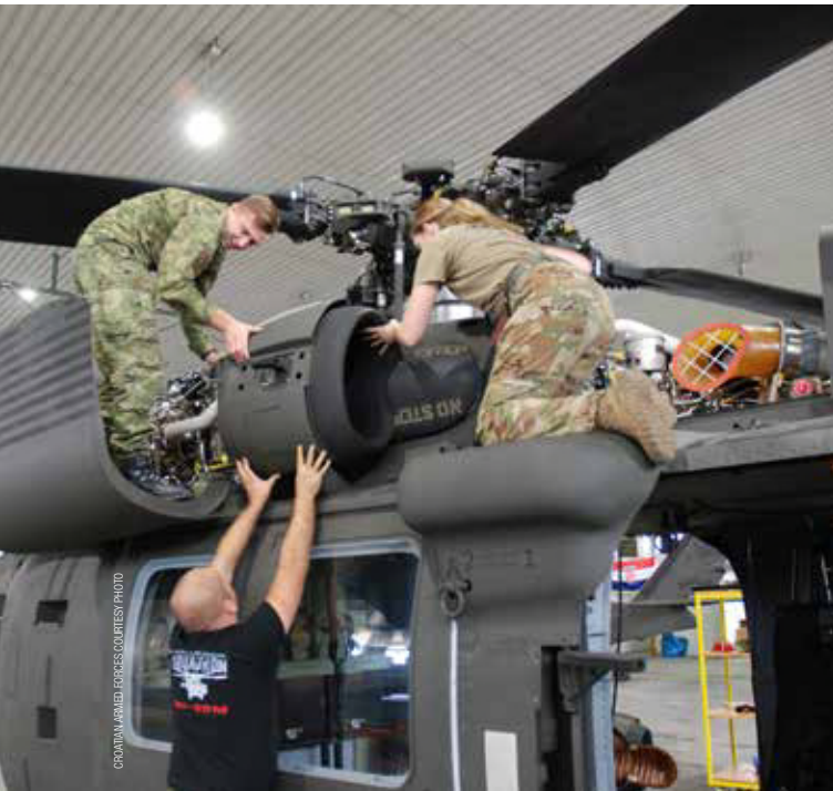
SGT Erynn Grochowski assists Croatian Armed Forces members to install an engine inlet on a UH-60M Black Hawk helicopter during a 120-hour inspection, during a skills exchange mission Sept. 17-30, 2022, in Croatia.
