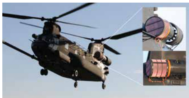
MH-47 with Engine Barrier Filter testing.
