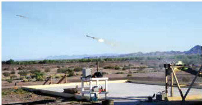
Hydra-70 M274 Smoke Signature-Practice Rocket being fired from M260 Rocket Launcher at Rocket Alley firing position at Yuma Test Center, AZ.
