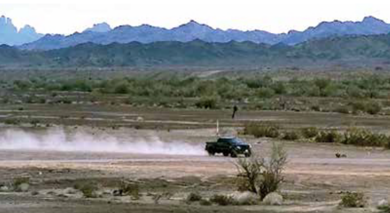
JAGM Engagement Before and After – Successful engagement of a Ford Raptor traveling at 77 mph and still accelerating. Test executed to stress the dual mode seeker performance and validate the pilot vehicle interface on the Apache.
