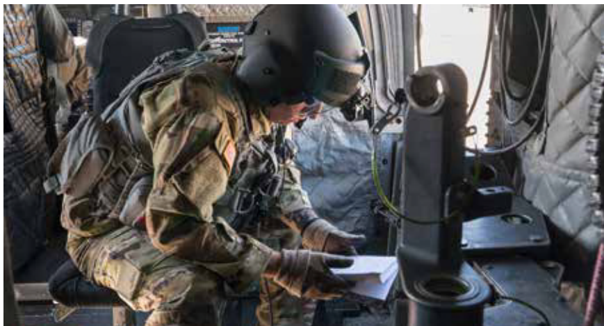
A crew chief from the 160th Special Operations Aviation Regiment (Airborne) conducts pre-flight inspections on an MH-47G Chinook helicopter.
