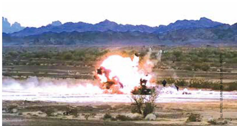
JAGM Engagement Before and After – Successful engagement of a Ford Raptor traveling at 77 mph and still accelerating. Test executed to stress the dual mode seeker performance and validate the pilot vehicle interface on the Apache.
