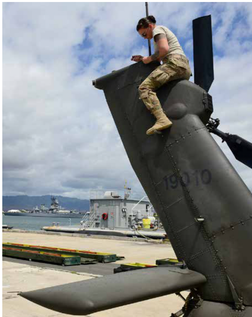
SPC Bethany Biryukova from the 25th Combat Aviation Brigade removes an antenna off an AH-64 Apache that landed at Joint Base Pearl Harbor-Hickam enroute to Wheeler Army Airfield.
