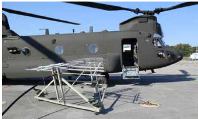
CH-47F undergoing Electromagnetic Vulnerability (EMV) testing at Redstone Test Center.
