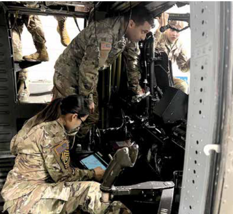
Left to right are PV2 Miranda, SGT Jones, and PFC Davis conducting UH-60 DAFCS troubleshooting.
