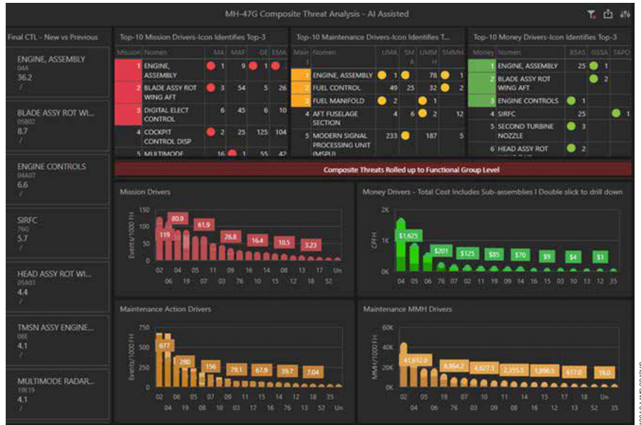
This picture represents a business intelligence tool used to identify Reliability, Availability and Maintainability, or RAM, data associated with mission, maintenance and money drivers. They provide leading indicators into our failure modes giving maintenance leaders the ability to apply the right resources against the right problems.
