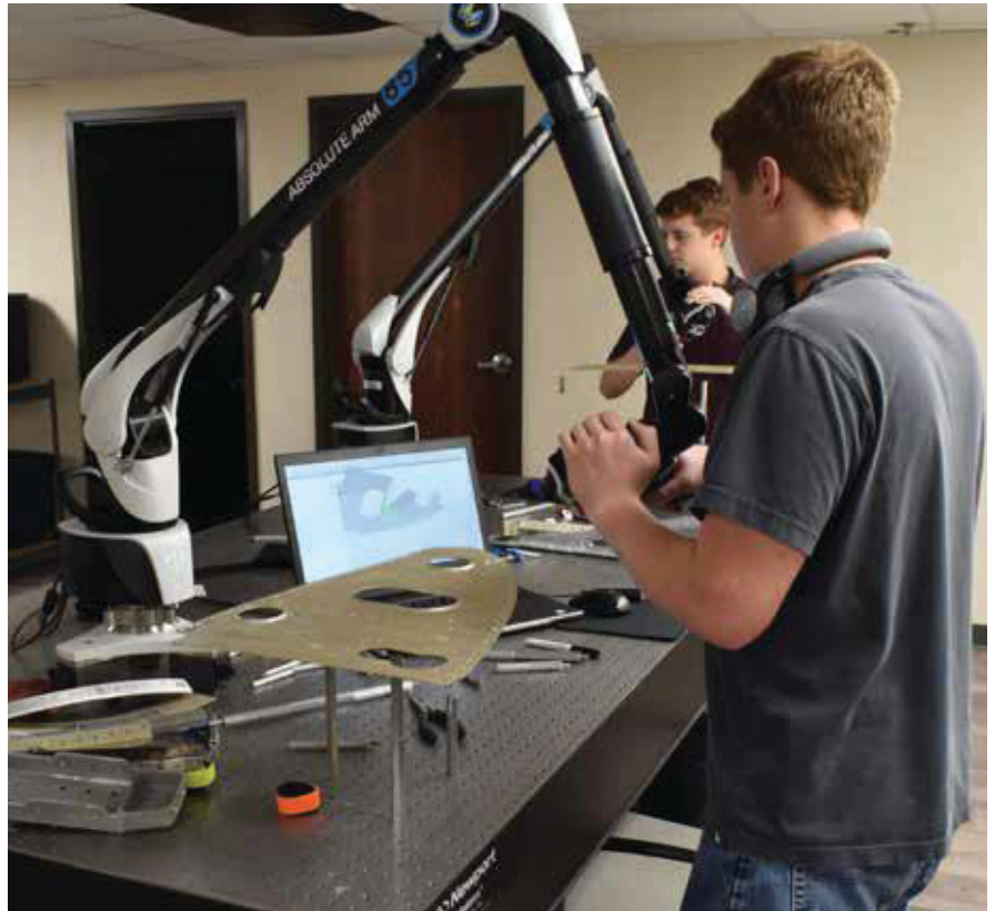
National Institute for Aviation Research personnel use high fidelity scanners during the reverse engineering of the UH-60L.
