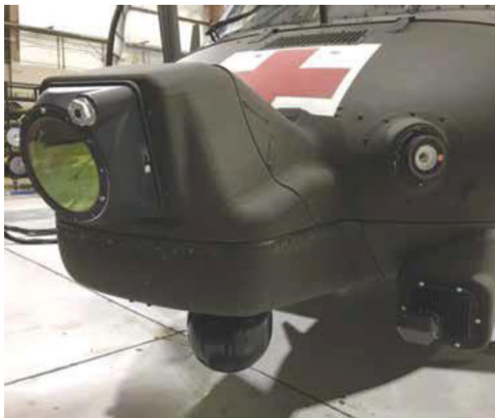
Light Detection and Ranging (LiDAR) Sensor and Infrared Camera installed on an HH-60M.
