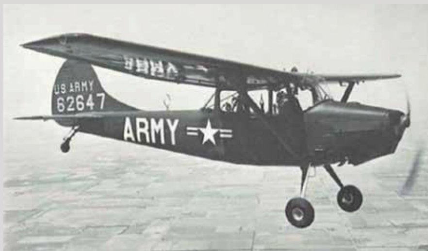
An O-1 (L-19) Bird Dog; a derivative of the Cessna 305, replaced the L-4 Cub and Stinson L-5 as the Army Ground Forces' cooperation aircraft; it would faithfully serve in two wars, Korea and Vietnam.
