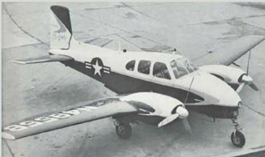
The L-23 Seminole, or U-8D/F, was built by Beech and was Army Aviation's first twin-engine fixed wing aircraft. This air taxi for staff personnel was a six-place type with a tricycle landing gear. Between 1952 and 1962, the Army procured 358 machines.
