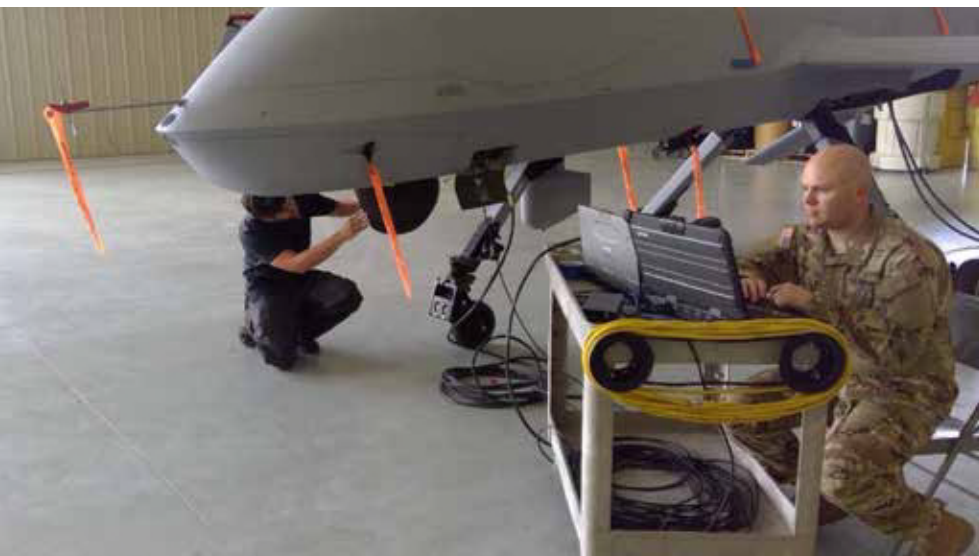
An MQ-1C Gray Eagle Maintainer (15M) and an Army Field Service Representative (FSR) work together to perform a diagnosis on a CSP through a portable workstation.
