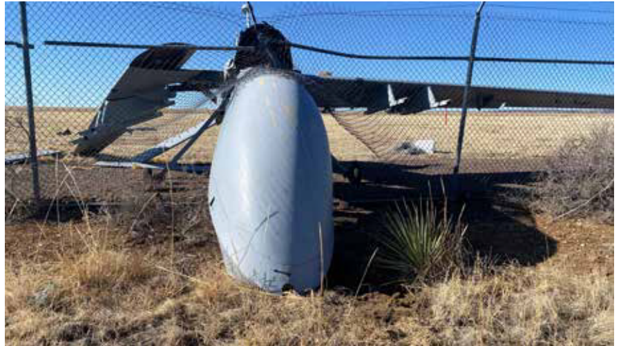
Individual failure led to the extensive damage pictured here of a Gray Eagle that was not deiced prior to attempted flight resulting in an overrun and fence impact.
