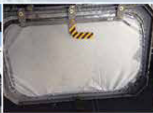
CH-47 INSIDE SHADES "HEAT SHIELDS" NSN: 1680-01-661-1895
