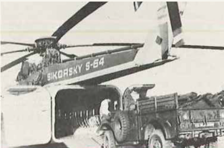
CH-54A pod for hauling equipment and vehicles
