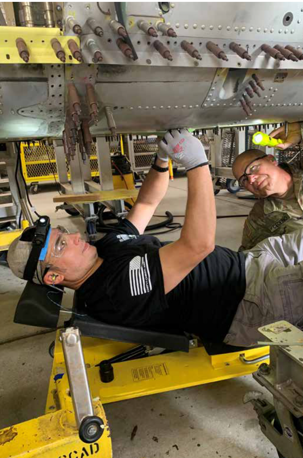
Depot artisan Jonathan Langford works on the lower outer skins of the Black Hawk fuel cell before primer and or sealant is applied, and rivets are permanently installed through aircraft structure. He is assisted by Pennsylvania National Guard SSG Asdrubal Cedeno, Eastern Army Aviation Training Site (EAATS).
