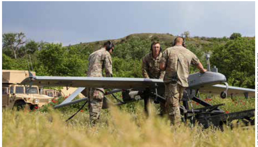
Soldiers assigned to the 7-17th Air Cavalry Squadron, 1st Air Cavalry Brigade perform routine maintenance on an RQ-7B V2 Shadow during Exercise Swift Response on May 10, 2022 at Krivolak Training Area, North Macedonia.
