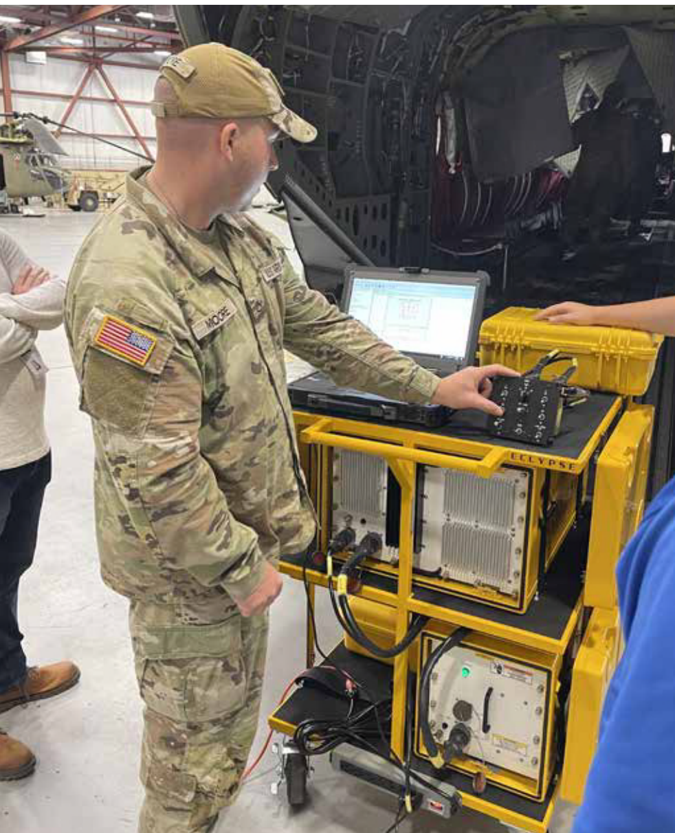
A 10th Combat Aviation Brigade technician runs a functional test on a panel next to a CH-47 helicopter with the Automatic Wire Test Set (AWTS) – Tests More Than Wiring.
