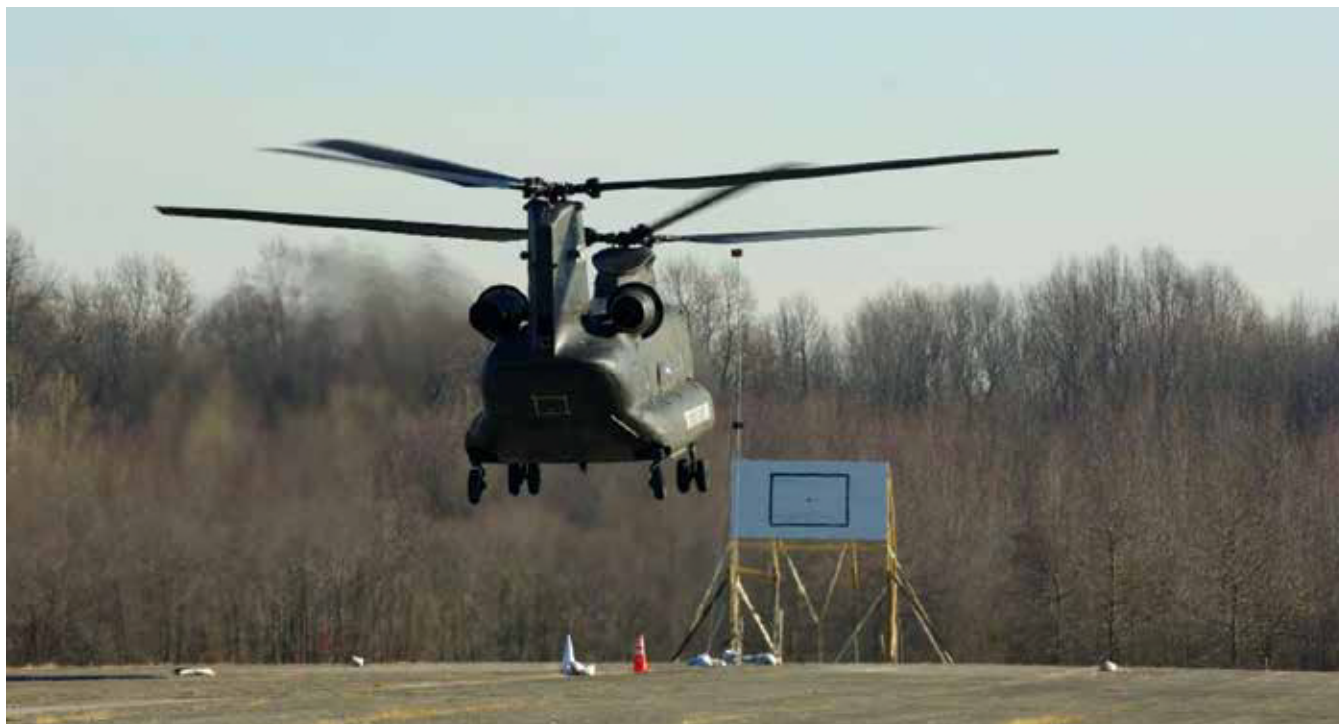
The CH-47F DAFCS development aircraft performing the ADS-33E Hover Mission Task Element Maneuver.
