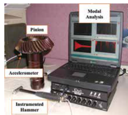
Figure 1. Rap test setup for measuring frequency response of a pinion gear.
