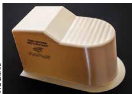
Left Top: A 3D-printed UH-60 External Electrical Connector Cover made using a digital scan. Using the digital scans of parts, Soldiers will be able to print their own replacement parts in forward-deployed areas.
