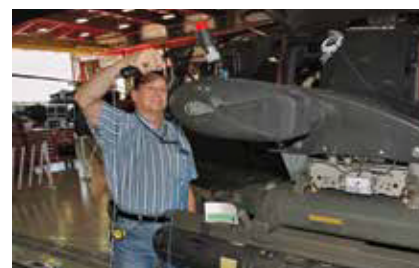
Figure 2. Rap test on an external store wing.
