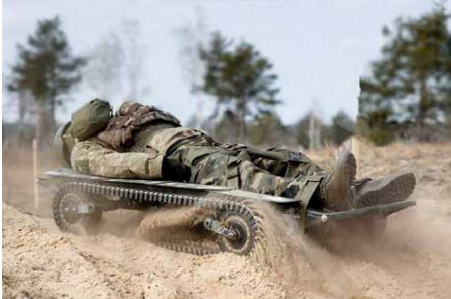
Example of ground robotics Ukrainian Defense forces are using for Casualty Extraction.
