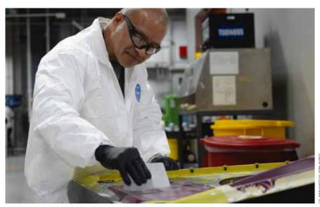
Composite Worker Sammy Cabrera repairs a UH-60 Black Hawk fuel cell panel, specifically a damaged aluminum honeycomb panel.
