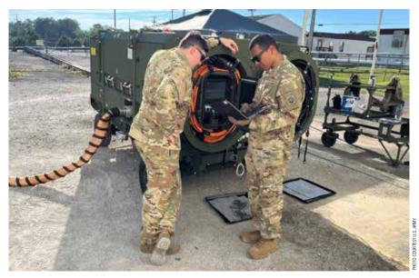
Soldiers verifying an air start work package during the AGPU 1.1 Logistics Demonstration on Redstone Arsenal, AL. Note the air start hose extending from the left side of the AGPU 1.1.
