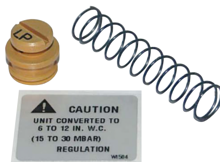
Regulator Conversion Kit, Natural Gas to LP
