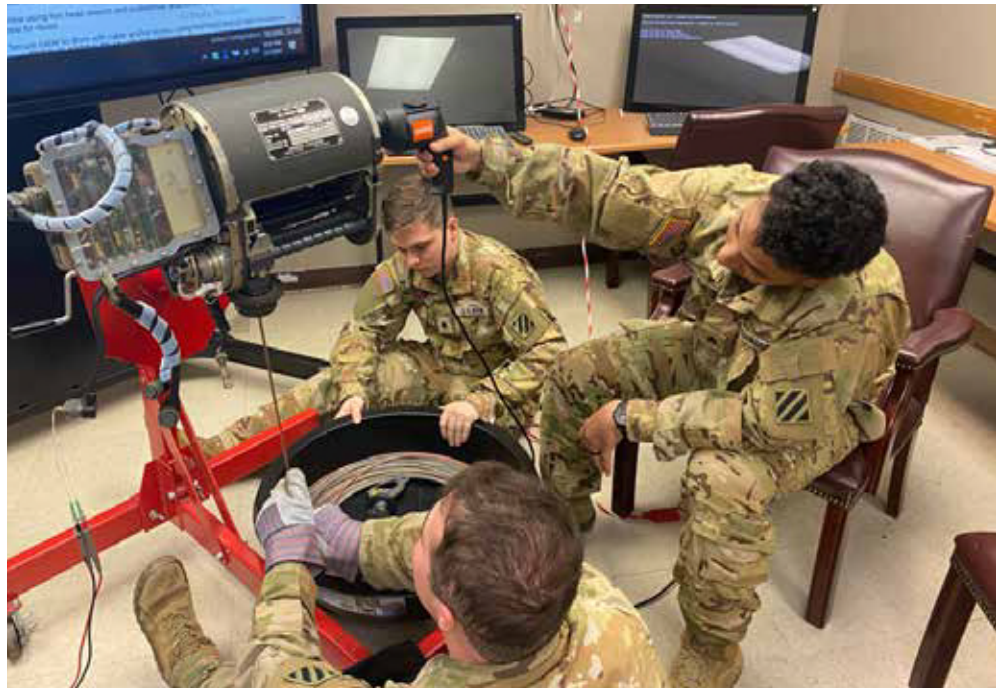
Students from C/2-3 conduct troubleshooting and maintenance tasks on the rescue hoist.
