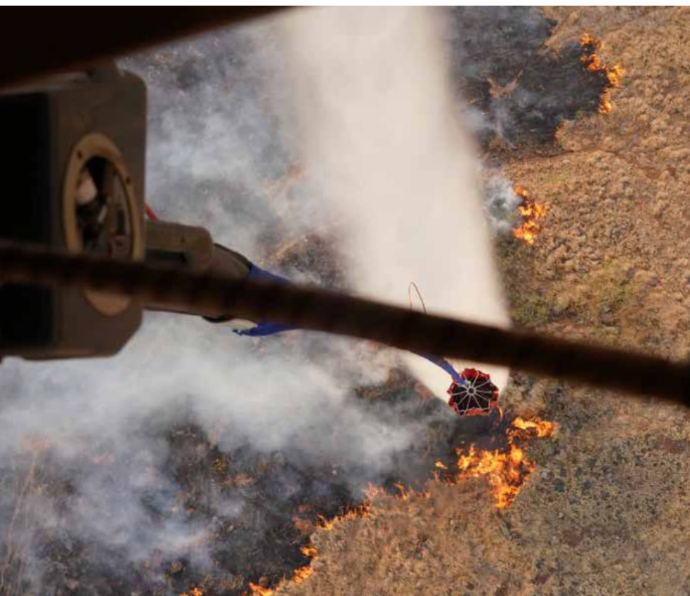
View from the CH-47 center cargo hook of HI-ARNG fighting fires in Maui using a 2,000 gallon waterbucket.
