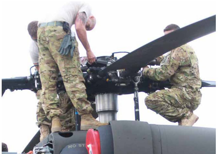
Soldiers from the 449th Combat Aviation Brigade inspect a UH-60 Black Hawk rotor system.
