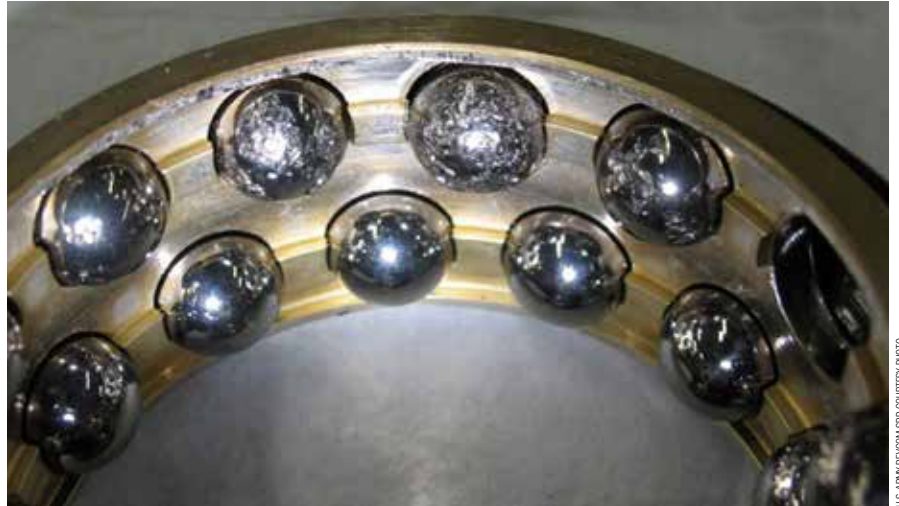
Apache nose gearbox failure.
