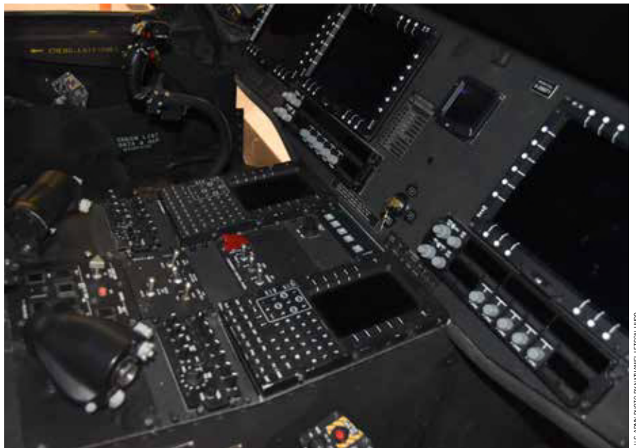
The UH-60V cockpit is fully digital and features an open system software architecture enabling efficient integration of future technology, upgrades, and integration of component alternatives.
