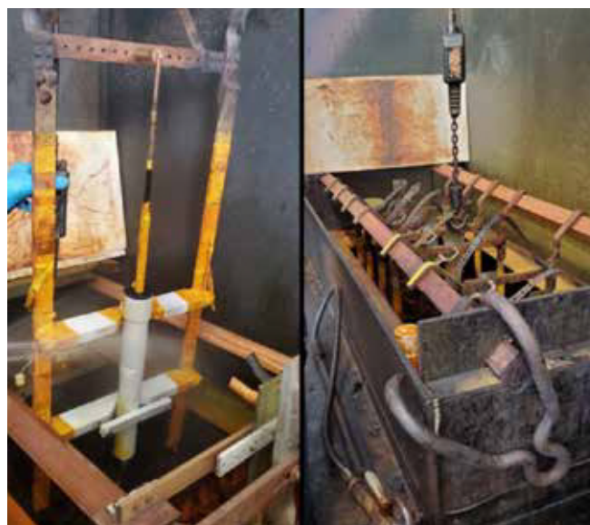
A two-bus bar chrome tank system for the plating process enables superior control and efficiency in chrome plating inner diameters.
