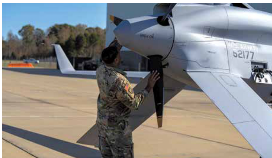
160th SOAR (A) Soldier conducts maintenance on MQ-1C.
