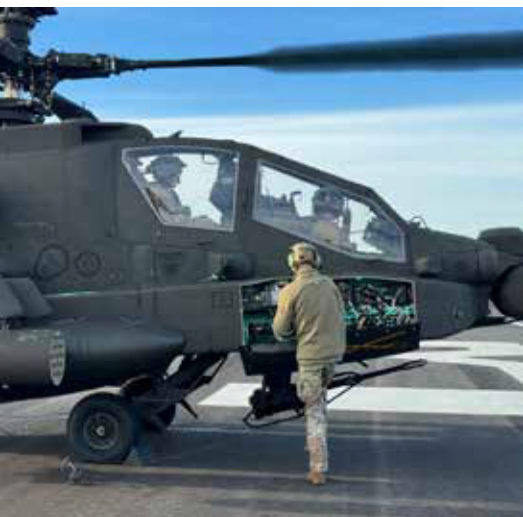
A Soldier from Co. B, 96th ASB, chalks the 30mm gun on an AH-64E prior to loading rounds in Monroe, Louisiana, Jan. 13, 2024.
