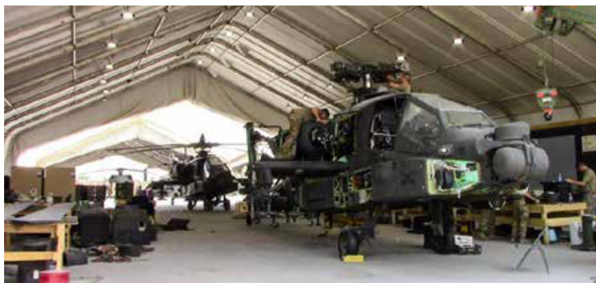
Left: Soldiers conduct a 500-hour Phase Maintenance cycle and upload an updated MDS on an AH-64E Apache. Above: One of many visits by ARAT-PO to support units around the country.
