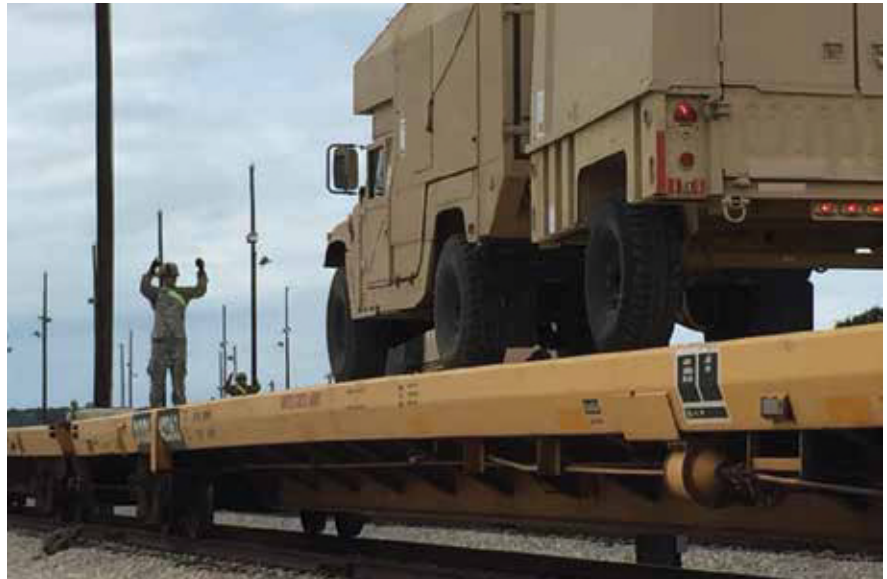
A U.S. Army National Guard Soldier provides safety and guidance at the Rail Operations Center at Fort Hood, Texas, as the equipment of the 449th Combat Aviation Brigade is loaded on the ramp Oct. 11, 2017.
