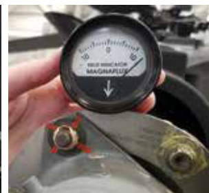
Magnetic field indicator showing abnormally high magnetism on tail rotor drive shaft of H-60M which had confirmed lightning strike
