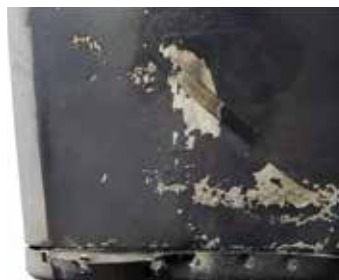
H-60M tail rotor blade with lightning strike damage
