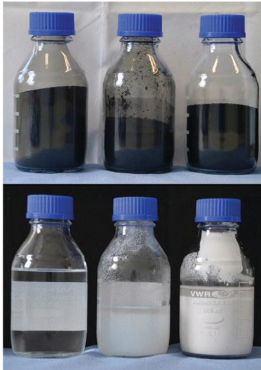
Top, primary product from left to right: raw rCB, clean rCB (96+), pearitized clean rCB (96+). Bottom, secondary products recovered from the ash, from left to right: liquid sodium silicate or "water glass", precipitated SiO 2 , precipitated ZnSO 4 .
