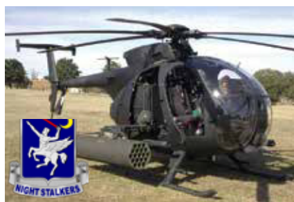
The OH-6 'Little Bird' has been constantly modified. Shown is an AH-6, sporting rockets and mini-guns.
