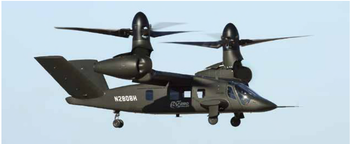
Bell Textron's V-280 Valor, a joint multi-role (JMR) technology demonstrator (TD), logged more than 200 flight hours during the FLRAA demonstration and risk reduction efforts to help Bell develop the future FLRAA model.
