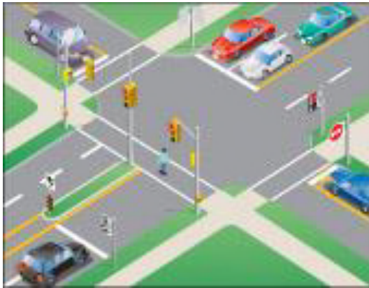
Figure 1: Intersection Pedestrian Signal (source: MTO)
