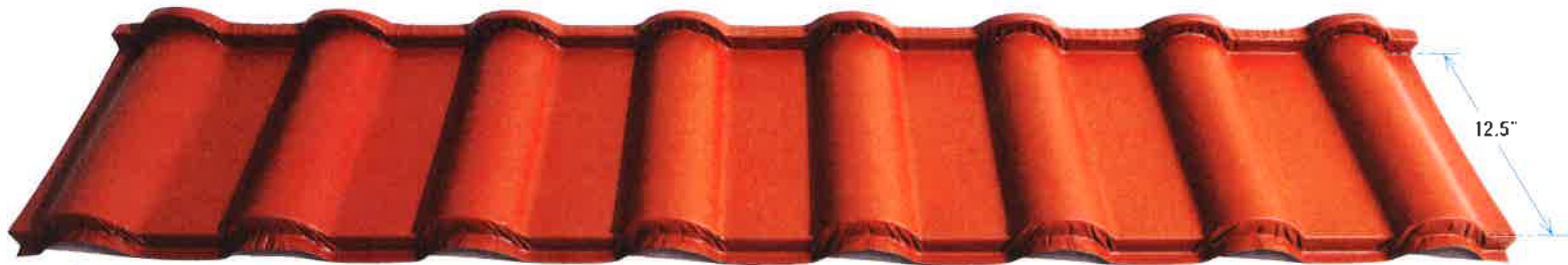
PVDF PRE-PAINTED GALVALUME (AZ 165) STEEL SYSTEM WITH KYNAR 500® RESIN ASTM-A792 SS GRADE "33" GAUGE: 29 (.017" THICK)
