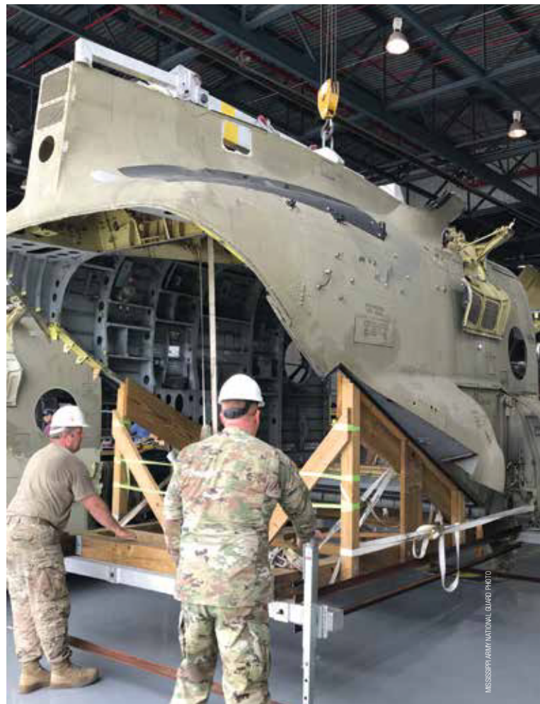
MSG Brandon Creel (right) Aircraft Maintenance Supervisor, and SGT Kevin Cooke (left) Sheet Metal Mechanic, Federal Military Technicians with Company A, 1108th TASMG, MSARNG move the aft section of a CH47F away from the airframe following an aircraft de-splice procedure.
